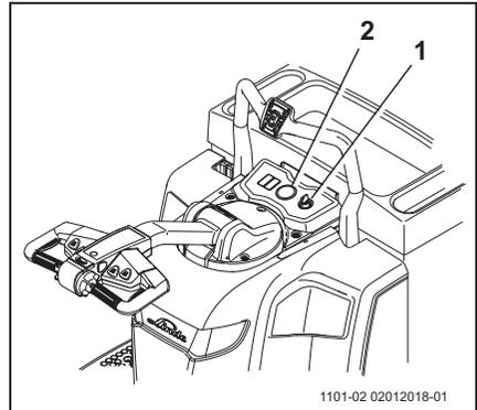
The truck is equipped with a static-return-to-neutral function. If the travel control is out of the neutral position at start-up, fault code t 307 will be displayed and the red fault indicator will come on. This fault may be cleared by releasing the travel control.
