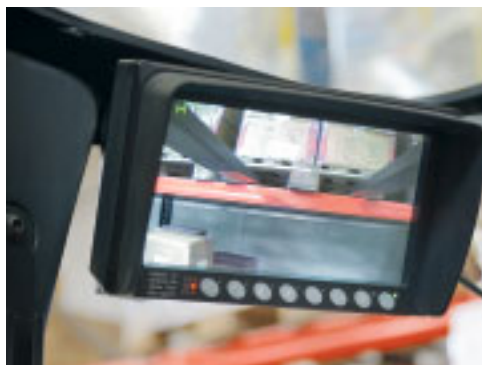
Vision package for improved visibility with innovative dual cameras mounted on overhead guard and mast
