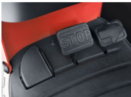
Optional single accelerator pedal version with selector switch on console to change travel direction. Left foot interlock switch
