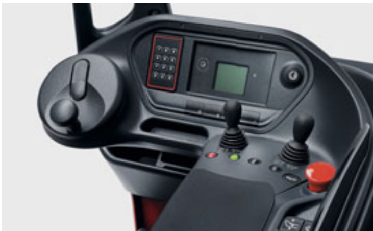
Responsive and precise finger-tip, joystick control of the mast functions
