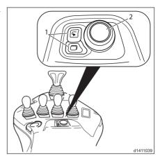
The Linde drive controller is operated using the rotary/push button (2), the "Back" button (1) and the "Switch" button (3).
