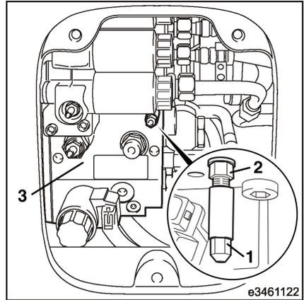
In order to access the manual lowering screw (1), the fan grill with its attached fan must be removed (see arrow).
