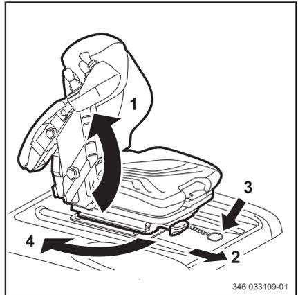
The battery cover may now be opened. To return the seat to the straight-ahead position, pull the chain again and rotate the seat. Ensure that the mechanism locks into the straight ahead position.
