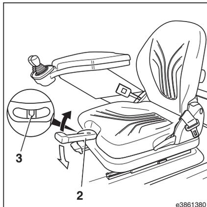
Pumping the lever (2) upwards adjusts the suspension to accommodate more weight.
