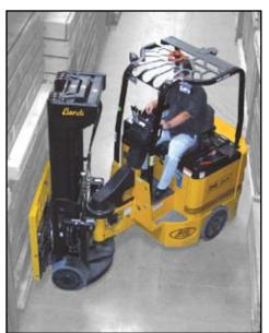
Awkward wide loads can also be handled effectively in narrow aisle using the 4-wheel Bendi with lift heights to 433-in (11M) and capacities to 4,500-lbs (2,045-kg).
