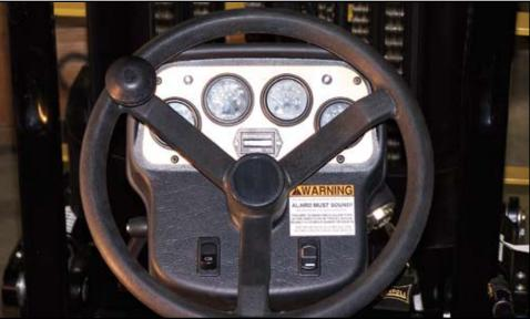
The LP Gas Bendi instrument cluster monitors all operational functions including: battery charge, engine coolant temperature, hydraulic oil temperature and oil pressure. An hour meter, low fuel indicator and filter replacement indicator are also standard.
