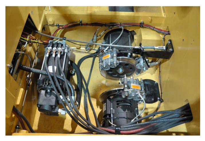
The Slotted Clevis on the Brake Master Cylinder Allows about 3" of free Brake Pedal Travel. As the Operator uses that free Pedal Travel, a Sensor Magnifies the Regenerative Braking Function of the Controller and Motors to Stop the Unit Electrically to Eliminate wear to the Brake Pads. Physical Brakes are used only in Accident Avoiding Stops.
