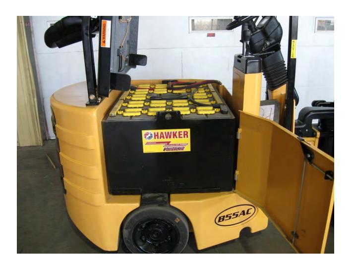
Model 24-85-23 - 48V - 935 AH - 43 KWH
