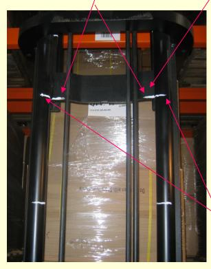
Raise inner mark 2" or 3" higher than outside mark = pallet Put Away lift height
