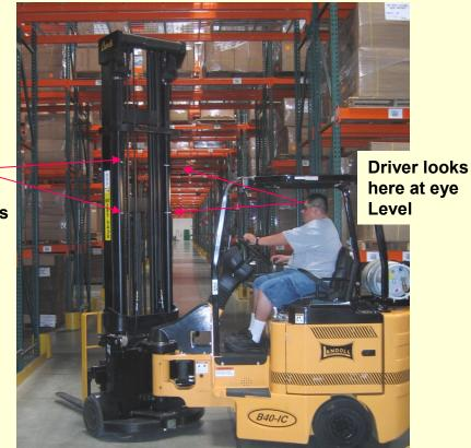
This Position = Top Pallet at Level Six Entry Indicator – Dead Vertical Center of Pallet Opening Every Time
