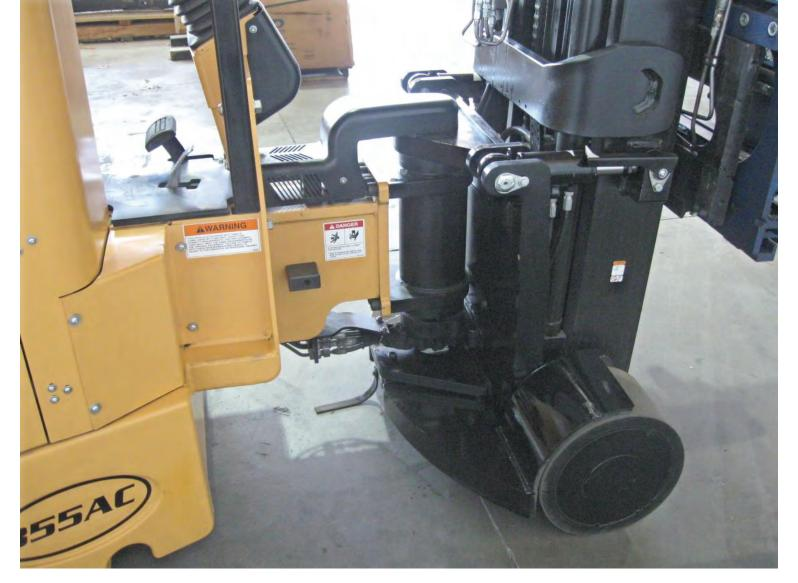
**Dura-Steer on Standard B55AC with Tilting Mast**
