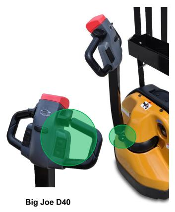
An AC travel controller enables the drive motor to deliver exactly the right mix of torque and speed needed by the operator resulting in smooth and accurate travel control.
