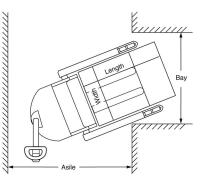
Aisle dimensions listed above assume the minimum bay width to be straddle OD plus 5" (2.5" on each either side of straddle leg). Truck performance may vary due to application requirements' and changes in model design.
