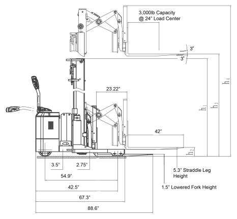
Overall length increased by up to 3" when control handle is perpendicular to the direction of travel
