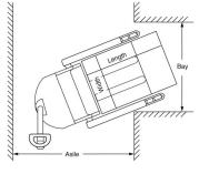
Aisle dimensions listed above assume the minimum bay width to be straddle OD plus 5" (2.5" on each either side of straddle leg). Straddle OD is the load width plus 8". Truck performance may vary due to application requirements' and changes in model design.
