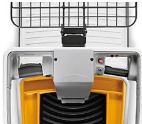
Crown: Left Hand Directional Toggle Right Hand Twist Grip Travel Control
