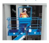
transfer the kinetic energy into surrounding structures while maintaining a protected area for the operator. The device can be attached to boom lifts with 6 ft. to 8 ft. platforms and allows for excellent visibility. It weighs 36 lbs. and is bolted directly on the boom lift's platform; no modifications are needed.
