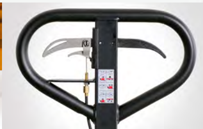
Travel direction selected by adjusting the handgrip on the towbar
