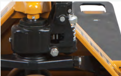
Greaseable bushings ensure a long service life
