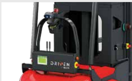
3D pallet detection via camera
