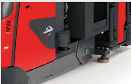
Real-time truck position detection
