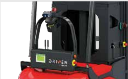
3D pallet detection via camera
