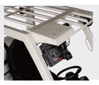
Extended Overhead Guard Extension provides protection to mounted components, including onboard computer and headlight (shown).
