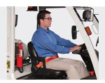
**High Visibility Seatbelt**Bright orange seatbelt provides instant visual confirmation that operators are maintaining this safety requirement.
