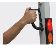
Reverse Assist Grip with Horn Provides operator control while driving in reverse. Keeps operator's hand inside the compartment for safer operation.
