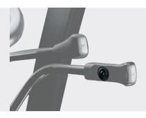
**Auto-Fork Leveling**Conveniently located on hydraulic lever, thumb-actuated button is used to automatically tilt the mast forward bringing the forks to 90° for easier load placement and retrieval operations.
