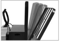
**Load backrests** have a slip-on or tilt down design available to facilitate battery change out. Tilt down includes Nissan's EZ release feature.
