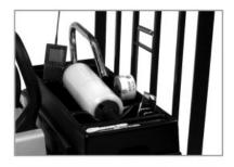
Magnetic convenience tray adheres to the top of the battery box. Includes shrink wrap holder and room for operator's tools.
