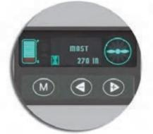
**Digital Fork Height Indicator** Fork height is displayed on the meter panel, giving operators a confidence boost while working in areas with high racking.
