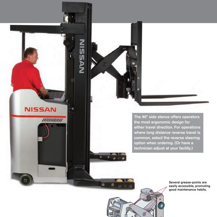
The SRX Series' reach mechanism incorporates canted roller bearings that travel within the bounds of the mast's "I" beam inner rail.
