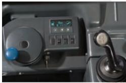
**Speed Sensing Steer Control** Operators experience a quicker response to their steering commands while the SRX is traveling at a faster rate. Conversely, this standard feature allows them to perform operations using slower, more precise movements when driving at a slower speed, such as while negotiating aisles or racking.
