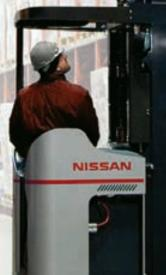
The SRX includes several standard features to help keep your operator secure while on the job, including an auto-mast lock, to disable hydraulic functions if the presence pedal is not depressed. There's also a high mast travel speed control, and an automatic applied parking brake which engages as soon as the SRX comes to a complete stop, return-to-neutral, and anti-rollback with ramp start.
