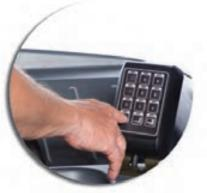
Automatic Fork Height Selector Save valuable time during storage and retrieval operations with six different fork height stop settings, for each of two rack types. Option includes Digital Fork Height Indicator.
