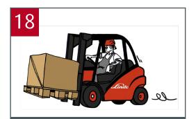
The driver must be in control of his/ her forklift at all times. Drive carefully with full concentration. Never leave the forklift with a load raised in the air.
