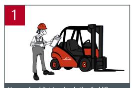
Use a checklist to check the forklift every day before starting work. Do not use a forklift that is damaged or not safe to operate.
