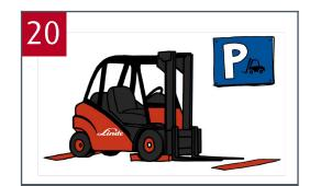
When parking the forklift in its allocated space, please remember the following instructions: lower the prongs, angle the forklift mast forwards, apply the parking brake and remove the key.
