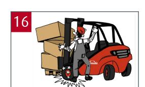
The forklift must only be operated from the driver's seat. All parts of the body must remain within the driver's cab. Never let your hands or feet dangle outside the forklift when driving.
