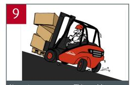
Never turn on a ramp. This could cause a serious accident, as the forklift could tip over and fall down. You must be particularly careful when driving on ramps.
