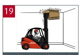
Never drive with a load high up in the air. It could fall and damage your environment and the goods.
