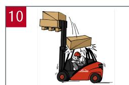
Ensure that the load is secured properly and do not transport anything at a height greater than the forklift's load protection grid. Falling goods could injure you and others.
