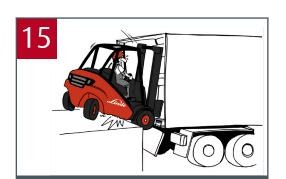
Think about load capacity when driving on contact plates. They must be capable of holding the forklift and the weight of the load. Contact plates must be secured sufficiently.
