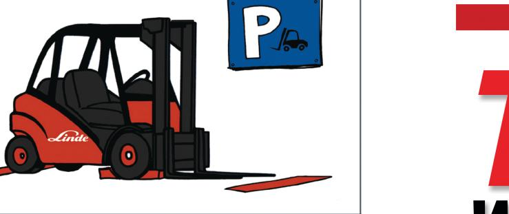
When parking the forklift in its allocated space, please remember the following instructions: lower the prongs, angle the forklift mast forwards, apply the parking brake and remove the key.
