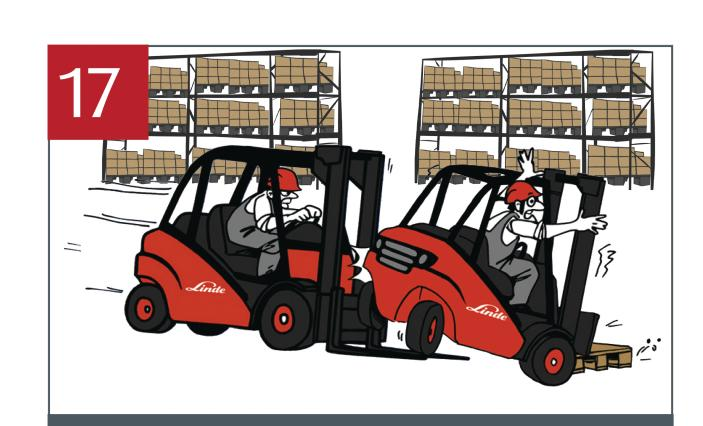
Keep at an appropriate distance from other forklifts, as you would when driving on the road. You must always maintain a safe braking distance.
