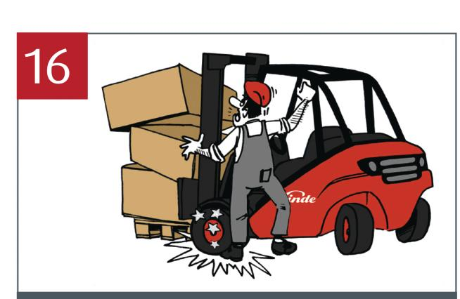
The forklift must only be operated from the driver's seat. All parts of the body must remain within the driver's cab. Never let your hands or feet dangle outside the forklift when driving.
