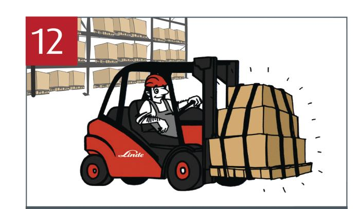
Make sure that the loads are stacked securely and are positioned in the centre of the forklift. Drive particularly carefully when you have a bulky load.
