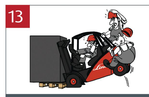
Never overload the forklift and do not add any additional weights. Never exceed the permissible lifting capacity, as this is a frequent cause of accidents.
