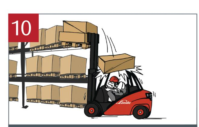
Ensure that the load is secured properlyt and do not transport anything at a height greater than the forklift's load protection grid. Falling goods could injure you and others.
