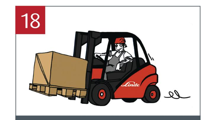
The driver must be in control of his/her forklift at all times. Drive carefully with full concentration. Never leave the forklift with a load raised in the air.
