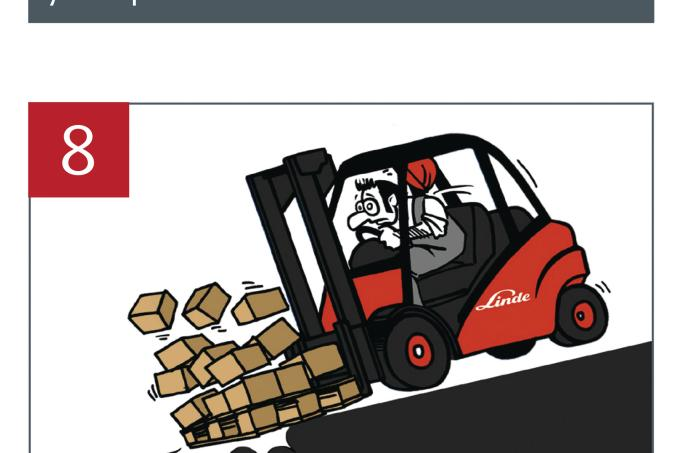
Always store the load at the front when driving up a ramp and at the back when driving down a ramp. Never drive downwards with the load at the front.
