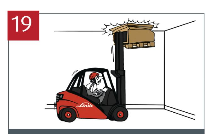
Never drive with a load high up in the air. It could fall and damage your environment. Look out for obstacles.
