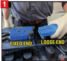
1 Disconnect BATTERY from TRUCK (Fixed End)
