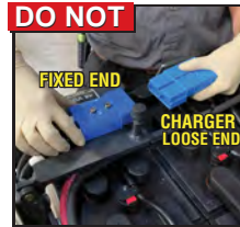
DO NOT Connect BATTERY to CHARGER to TRUCK (Loose End to Fixed End)
