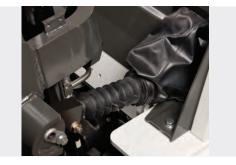
**Tilt Cylinder Protection** Cylinder boots and covers provide extra protection against contaminants that can cause premature wear on cylinder packing.
