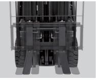
**Sideshifting Fork Positioner** Hydraulically positions forks, eliminating
