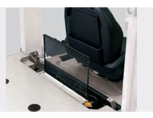
Radiator Screen Minimizes debris entering radiator, resulting in more efficient engine cooling.
