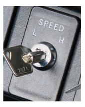
Select the security key switch option to lock in a pre-set high or low speed\*.
