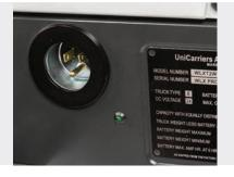
**Charger Unit** Sealed built-in battery charger option simplifies on-board battery charging.
