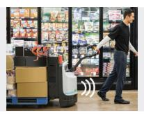
**Travel Alarm** Audible alarm may be preprogrammed for operations with: forks forward, forks trailing, or both.
