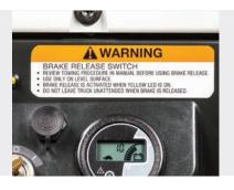
**Drive/Tow Switch** Electronically releases the parking brake to allow a disabled truck to be moved to a charging station or service area.
