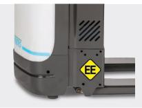
**U.L. Type EE Rating** Fire safety rated truck for applications requiring Type EE trucks, in accordance with NFPA 505 "Fire Safety Standards for Powered Industrial Trucks"
