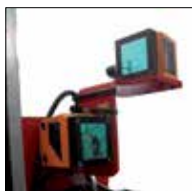
① Laser detector Laser sensor for upper row to detect presence of boxes in the upper part of the pads.
