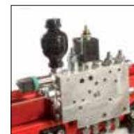
③ Proportional valve Commands the hydraulic pressure in the clamping cylinders.
