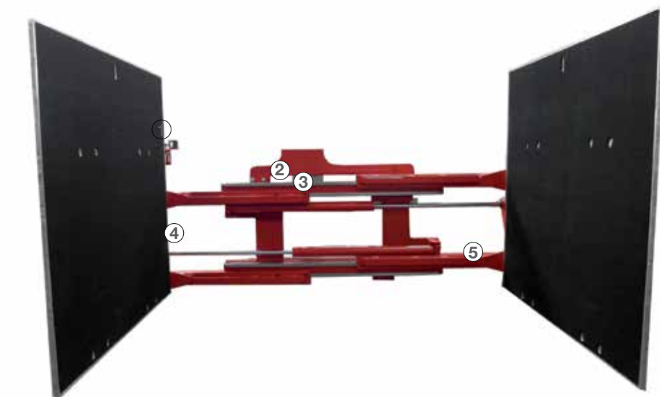
① Laser detector Laser sensor for upper row to detect presence of boxes in the upper part of the pads.
