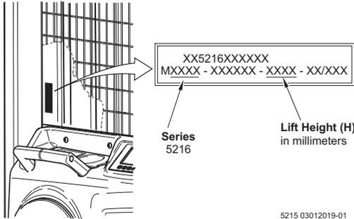
Mast heights are listed by lift height from the floor (H). This number is found in the mast identification code as shown above. Mast height dimensions in inches are rounded to the nearest 1/2 inch conservatively, ie h1 and h4 are rounded up; H, h2 and h3 are rounded down. Metric mast height dimensions (mm) are design values.
