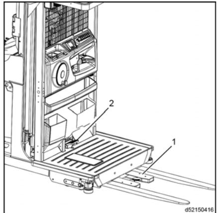
To unload the forks, the pallet must be in contact with the floor and the clamp released by pressing the release pedal (2). The truck may then be driven away from the pallet.
