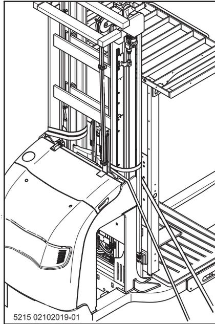
the truck and two at the rear, and position the remaining blocks in pairs on the right and left of the truck. The tension belts must be guided around the mast uprights on each side and securely attached to the transport vehicle.
