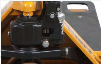
Greaseable bushings ensure a long service life
