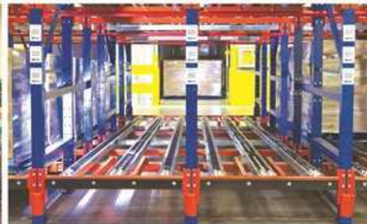
PALLET FLOW SYSTEMS FOR INVENTORY WITH EXPIRATION DATE
