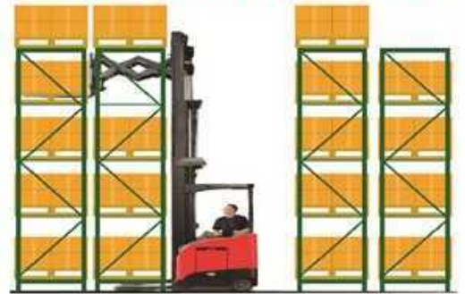
DOUBLE DEEP RACKING DOUBLE RACK = DOUBLE INVENTORY VOLUME!
